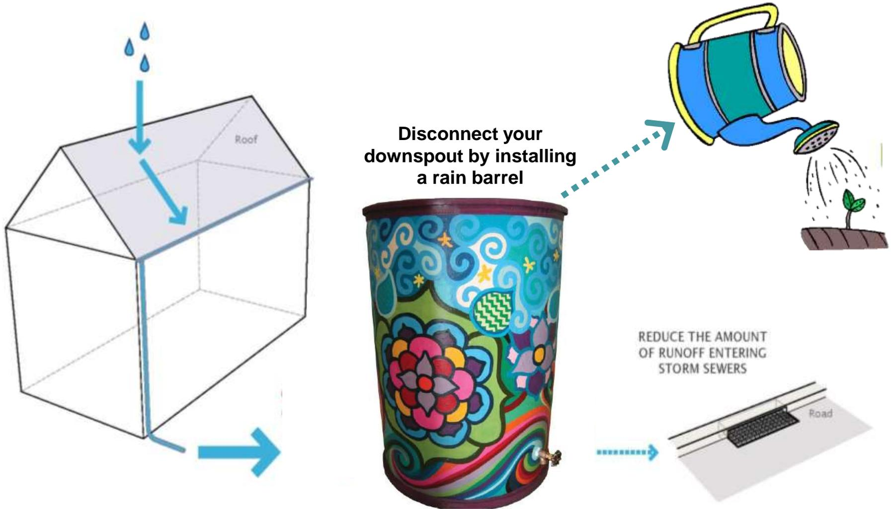
Impervious area is now **"disconnected"** from flowing directly into the storm sewer system
