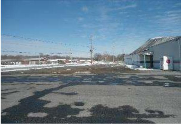
Grass pavers could be installed along the western edge of the building to treat its runoff. The parking lot could be retrofitted with bioretention islands and porous pavement. A preliminary soil assessment for this site suggested that the site's existing soils have suitable drainage characteristics for green infrastructure.
